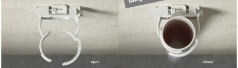
Size-accurate mounting of conduits from 16–50 mm! The conduit can be easily pre-fixed and by the push of a thumb you have a closed clip including drop protection.
